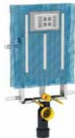
Kombifix Concealed Cistern for Wall Hung WC 1090 mm for Installation in Part-Height or Room- Height Pre-wall Installations with Fastening Material with Net for Plastering Thickness 80 mm
