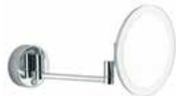
Wall Mounted Double Arm Mirror Magnifying x 3 LED Illuminated Mains Operated, 220 - 240 V, IP44 Concealed Connection with Progressive Switch with Dual LED Temperature Colour 220 x 140 (max 400) x 200 mm
